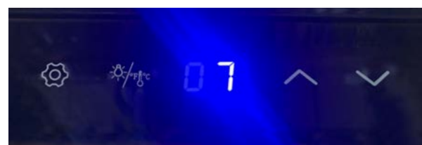
Digital touch screen thermostat / Termostato digitale con touch screen (+5°C +18°C)
